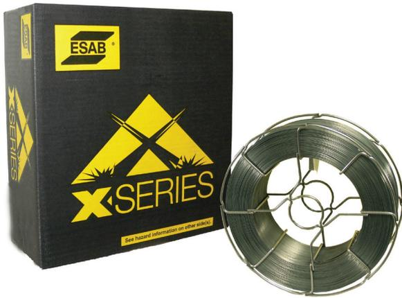
Dual Shield 710X is an all-position flux cored wire for general purpose welding. It provides outstanding operator appeal with an easily controlled arc, improved operation at both lower and higher current levels, minimal spatter and easily removed slag. Dual Shield 710X is designed primarily to be used with 100% CO<sub>2</sub> gas mix, especially for applications where weld joint restraint is high. Applications include railcars, barges, civil construction, light equipment and general fabrication.
